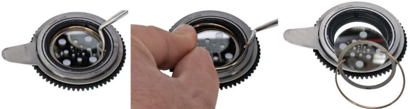
Locate the tab of the spring, and with a precision pick (or similar tool), carefully press the retaining spring inward to relieve the tension. Remove the retaining spring and carefully separate the GOBO from the GOBO Holder. Lastly, remove the flat washer attached to the removed GOBO and attach it to the desired replacement GOBO. Install the replacement Rotating GOBO following the steps above in reverse order.
